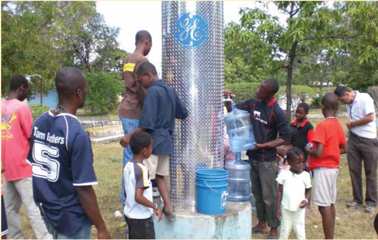
Above: The GE SunSpring at work at the SOS Children's Village in Santo, Haiti. Right: The SunSpring can produce 5,000 gal of safe drinking water per day.
