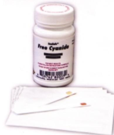
The SenSafe Cyanide test strip does not require any chemical mixing for detecting free cyanide levels in water down to 0.1 ppm. Simply collect a 50 ml sample, dip the strip into the water for 90 seconds, remove and match to the closest color to determine the concentration of free cyanide.
