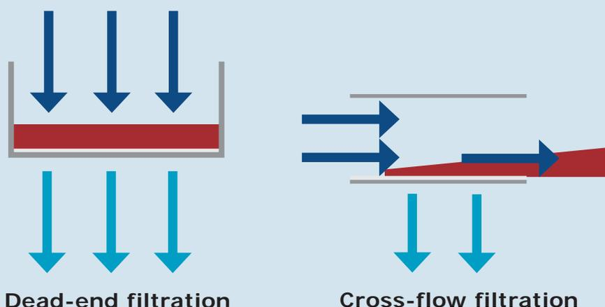
Figure 4. Cross-Flow Filtration
