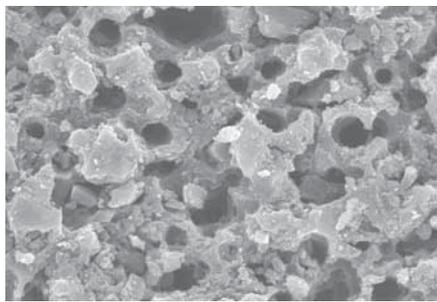
Figure 1. The microporous structure of activated carbon.
