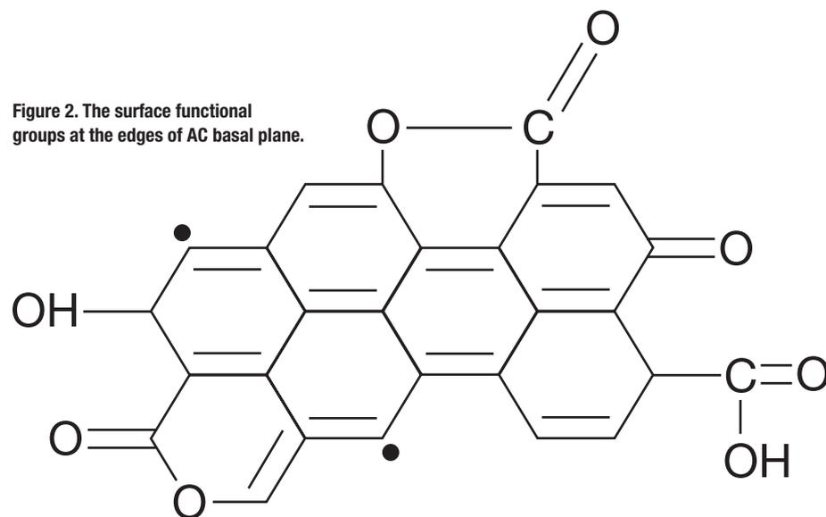
Figure 2. The surface functional groups at the edges of AC basal plane.
