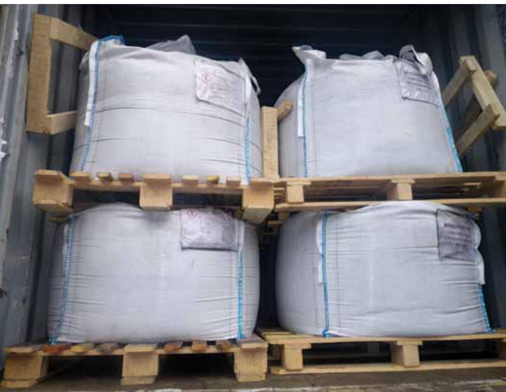
Solid manganese dioxide media, such as Pro OX, pictured here, contain a higher percentage of manganese dioxide than coated iron filter media.
