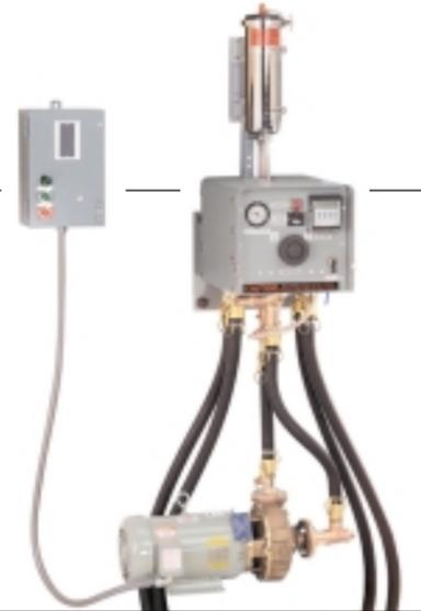
bromine feeder is used to treat potable water by adding a predetermined quantity of bromine to the desalinization system discharge line. The quantity of bromine added is contingent upon the seawater intake to the ship's water maker. If the seawater intake is considered noncontaminated, the low feed
