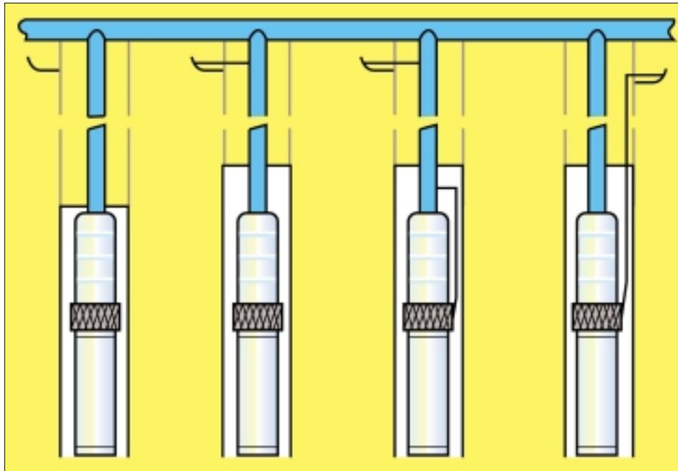
*Multiple pumps feeding a common supply manifold. This is a prime cause of water hammer.*
